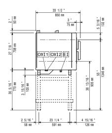
Cold Water inlet 1 CWI2 Cold Water Inlet 2 D Drain
